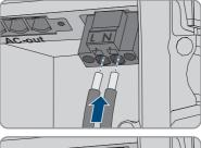
13. Ensure the conductors are plugged into the terminal points (round openings) as far at is will go and not into the actuation shafts (rectangular openings).
