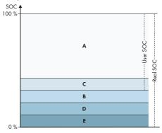
Figure 7: State of charge ranges of the battery in battery-backup systems
