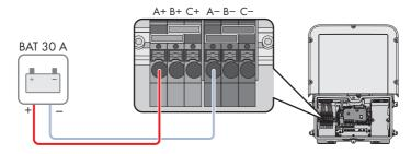
The battery must be connected to the terminal blocks A+ and A-.
