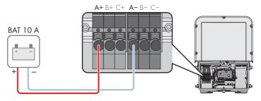
Figure 14: Overview for connection of one battery with a charging/discharging current limit of 10 A
