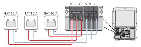
Figure 16: Overview for connection of three batteries with a charging/discharging current limit of 10 A each
