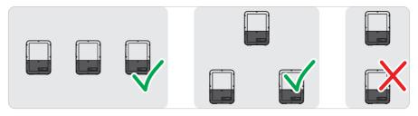
Figure 9: Permissible and impermissible mounting positions of multiple inverters
