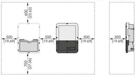
Figure 11: Recommended clearances(Dimensions in mm)
