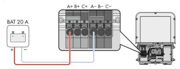
Figure 18: Overview for connection of one battery with a charging/discharging current limit of 20 A
