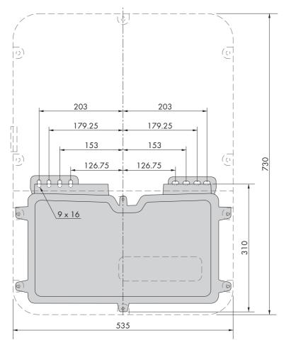
Figure 10: Position of the anchoring points(Dimensions in mm)
